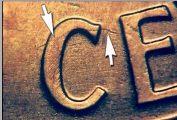
Die crack through upper letter "C" of CENT.
